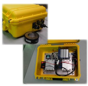
Dynamic measurement of bolt tension on a rotating Ball Mill: The Logger is mounted on the Ball Mill as it rotates at around 6-8 RPM, and is used to verify the dynamic load on critical bolts immediately following maintenance. It logs four or more channels of dynamic strain, plus one channel of inclinometer, at 100 Sa/s/Ch.
