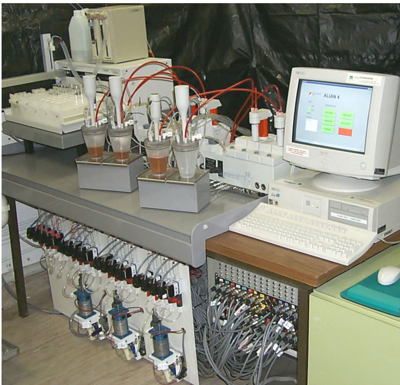
Fig. 1 – The working system, showing the control PC, Gilson Autosampler and Syringe Diluter, two Mettler Titrators and their associated beakers, the switch box, and piston pumps.
